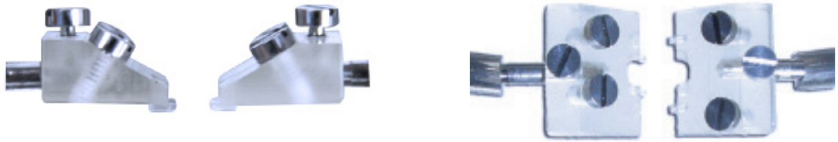
Figure 2.2 Illustration of correctly aligned supports of the Confocal Wire Myograph special designed jaws - view from the side (left) and view from the top (right)
