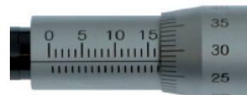
Figure A2.3 Example 2: reading = 16780 \mu\text{m}
