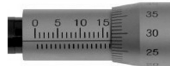
Figure A2.3 Example 2: reading = 16780 \mu\text{m}
