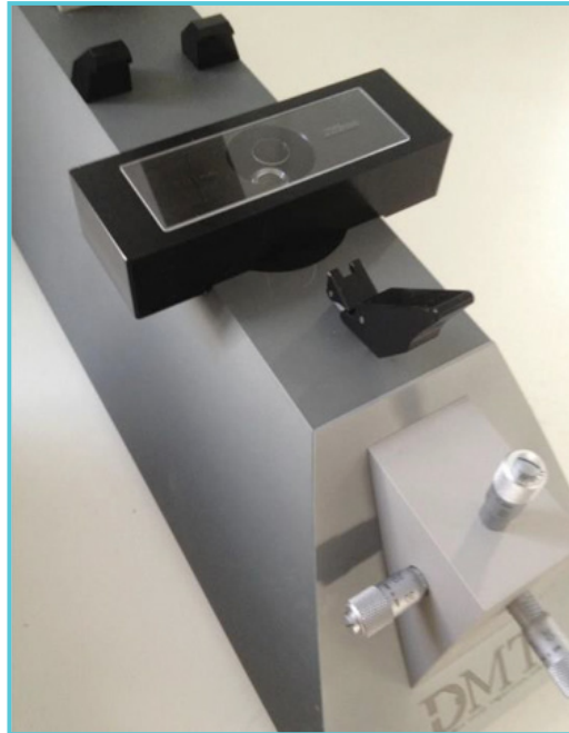
Figure 2.3 Place the micrometer positioner ruler on DMT Inverted Microscope
