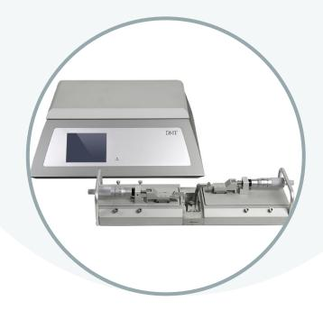
The Dual Wire Myograph System - 420A is designed for simultaneous testing of two vessels with diameters of  $30 \ \mu m$  - 3 mm, independently. The vessels are mounted as ring preparations by threading them over two parallel wires and securing the wires to two supports or "jaws". One support is attached to a precision micrometer, allowing manual control of vessel circumference and stretch. The other support is attached to a force transducer for measurement of force/tension development.
