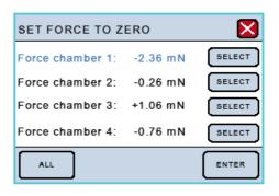
Once the desired setting has been chosen, pressing "ENTER" will lock the selection and be stored in memory. Pressing the white "X" in the red box will exit that menu and take you automatically to the Actual Force Display.
