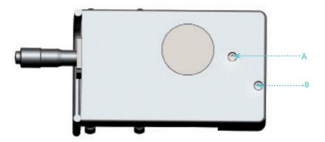
Figure 4.9 - The 2 screws that secure the transducer house to the chamber
